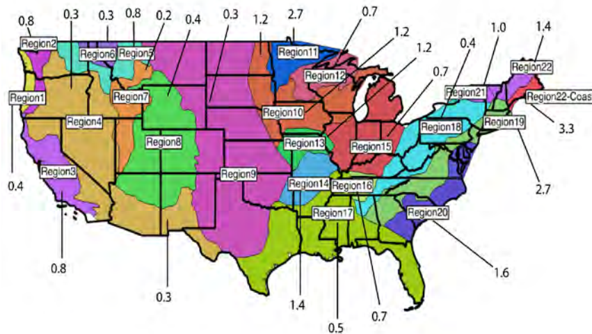
Figure 8: Updated \beta scaling factors for calculating geoelectric fields used in GMD vulnerability assessments based on newly available MT information
